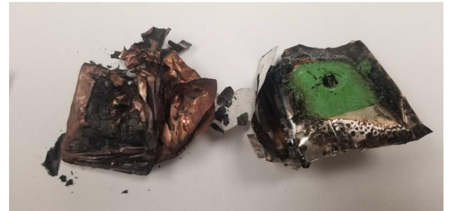
Standard pouch cell is destroyed in nail penetration test
